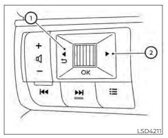
To change the status of the driving aids, use the ① or **②** button to navigate the settings screen. For additional information, see "How to use the vehicle information display" (P. 2-22) or (P. 2-46).
