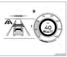
System set display with no vehicle détected ahead (12.3 inch (31.2 cm) display)
