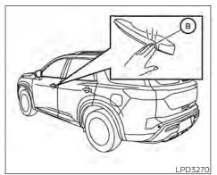
If a door handle is pulled while unlocking the doors, that door may not be unlocked. Returning the door handle to its original position will unlock the door. If the door does not unlock after returning the door handle, touch the door handle lock sensor to unlock the door.
