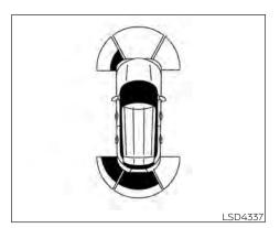
When the vehicle moves closer to an obstacle, the sonar indicator (detected area) appears in the vehicle information display.
