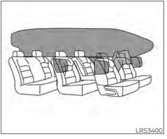
FRONT, 2ND ROW OUTBOARD, AND FRONT CENTRAL (if so equipped) SFAT-MOUNTED SIDE-IMPACT SUPPLEMENTAL AIR BAG AND **ROOF-MOUNTED CURTAIN** SIDE-IMPACT AND ROLLOVER SUPPLEMENTAL AIR BAG SYSTEMS
