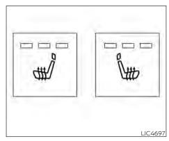
The 2nd row outboard seats are warmed by built-in heaters. The switches are located on the rear of the front center console and can be operated independently of each other.
