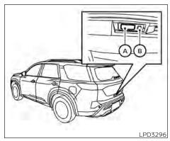
Liftgate opener switch and request switch
