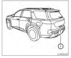
To display the rear view, the Rear View Monitor system uses a camera located in the rear bumper  $\bigcirc$ .
