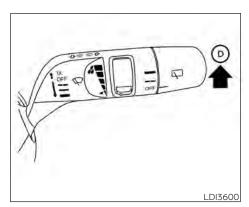
7. Finally, lift the windshield wiper and washer lever to the mist position (1) once and release. This action will cause the wipers to resume the set position.
