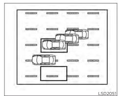
Illustration 10: - Entering from the side Illustration 10: The I-BSI system will not operate if your vehicle is on a lane marker
