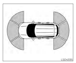
The sonar system sounds a tone to inform the driver of obstacles around the vehicle using the sonar sensors located in the front and rear bumpers...
