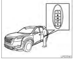
touch the lock sensor within 2 minutes to unlock all doors (B).
