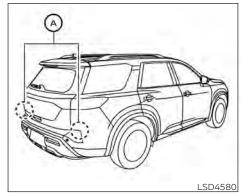
The RCTA system uses radar sensors (A) installed on both sides near the rear bumper to detect an approaching vehicle.
