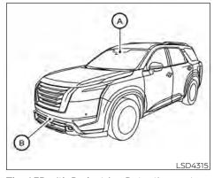
The AEB with Pedestrian Detection system uses a radar sensor located on the front of the vehicle (B) to measure the distance to the vehicle ahead in the same lane. For pedestrians, the AEB with Pedestrian Detection system uses a camera installed behind the windshield (A) in addition to the radar sensor
