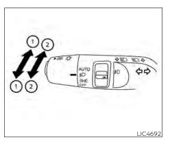
Move the lever up or down until the turn signal begins to flash, but the lever does not latch, and release the lever. The turn signal will automatically flash three times.
