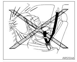
Even with the NISSAN Advanced Air Bag System, never install a rearfacing child restraint in the front seat. An inflating front air bag could seriously injure or kill your child. For additional information, see "Child restraints" (P. 1-34).
