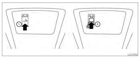
The Emergency call (SOS) button is used in combination with a NissanConnect® Services subscription to call for assistance in case of an emergency.
