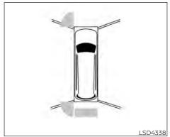
The sonar indicator also appears on the camera view of the center display.
