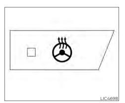
Push the heated steering wheel switch to warm the steering wheel after the ignition switch is placed in the ON position. The indicator light will come on.
