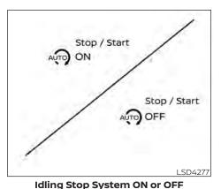
If the Idling Stop System is activated or deactivated using the Idling Stop OFF switch, the message is shown.
